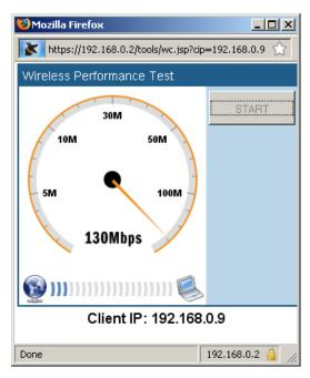
SpeedFlex' is a unique wireless performance test tool integrated within Ruckus Smart/OS that measures the Wi-Fi throughput of associated wireless LAN (WLAN) clients and can be invoked directly from the controller.
