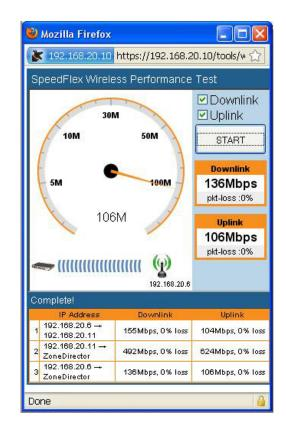
SpeedFlex<sup>TM</sup> is a unique wireless performance test tool integrated within the ZoneFlex<sup>TM</sup> family of centralized controllers that measures the Wi-Fi throughput of associated wireless LAN clients.
